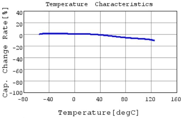
GCM155R71H333KE02 C-Temp. capchange, DC0.0V,
