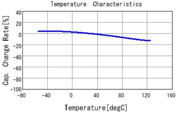
GRT033R71A103KE01 C-Temp. capchange, DC0.0V, AC1.C
