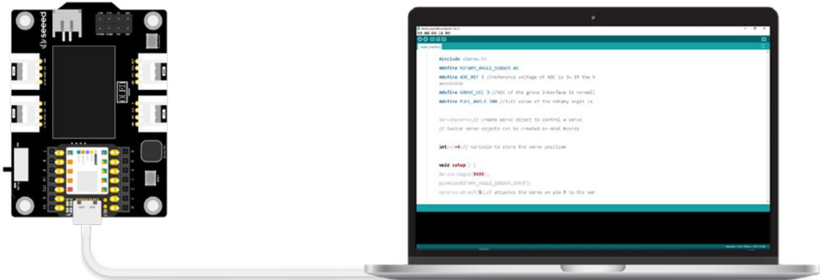
Next, click “Verification button” to verify the program. If verification is correct, click “Upload” button to upload the program to the hardware. When “Done uploading” is displayed in the debugging area, we can press the button to test if the LED light will light up.
