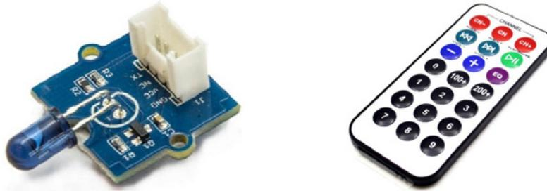
In a nutshell, the principle of infrared transmission and reception is that the input signal from the infrared transmitting end is amplified and then sent to the infrared transmitting tube for final transmission, and the infrared receiving end receives the infrared signal and is processed and reduced to an electric signal by the amplifier, thus realizing infrared control. If you want to learn more about "how does Infrared Communication work", please refer to the following articles:
