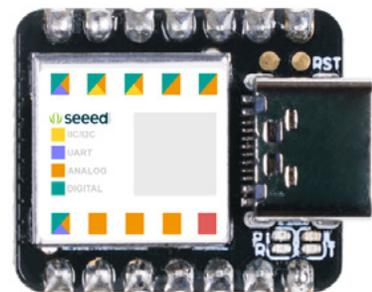
Seeeduino XIAO has 14 GPIO PINs, which can be used for 11 digital interfaces, 11 mock
