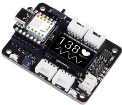
In order to make it easier and faster through Seeeduino XIAO to build the project, we are equipped with a powerful expansion board with rich peripherals on board, and can quickly connect more electronic modules to realize various functions. The expansion board leads out all the pins of XIAO, and the pin diagram is as follows:
