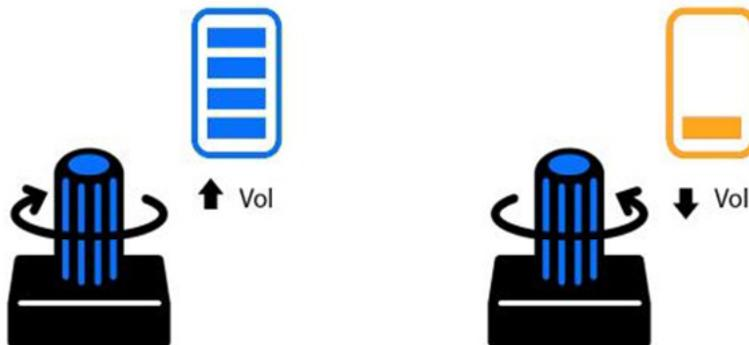
The knob potentiometer produces an analog output value between 0 and VCC on its connected pin. By rotating the knob, the output voltage can be changed. the angle range of the knob is 300 degrees,and the output value is 0–1023.We can control the LED lamp to produce a brightness change by the knob potentiometer,and also control the steering engine to rotate at different angles, etc.
