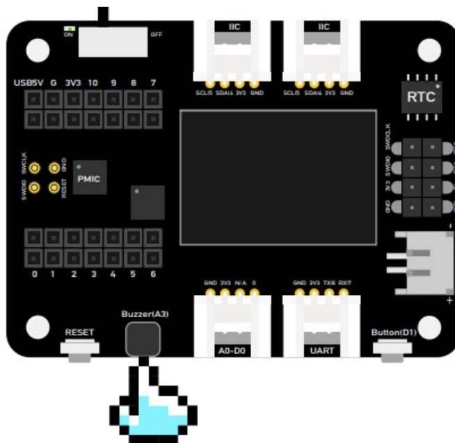
In the Seeeduino XIAO expansion board, there is an onboard passive buzzer connected to the A3 pin, to which we can output PWM waveform pulse signals to control the buzzer sound.
