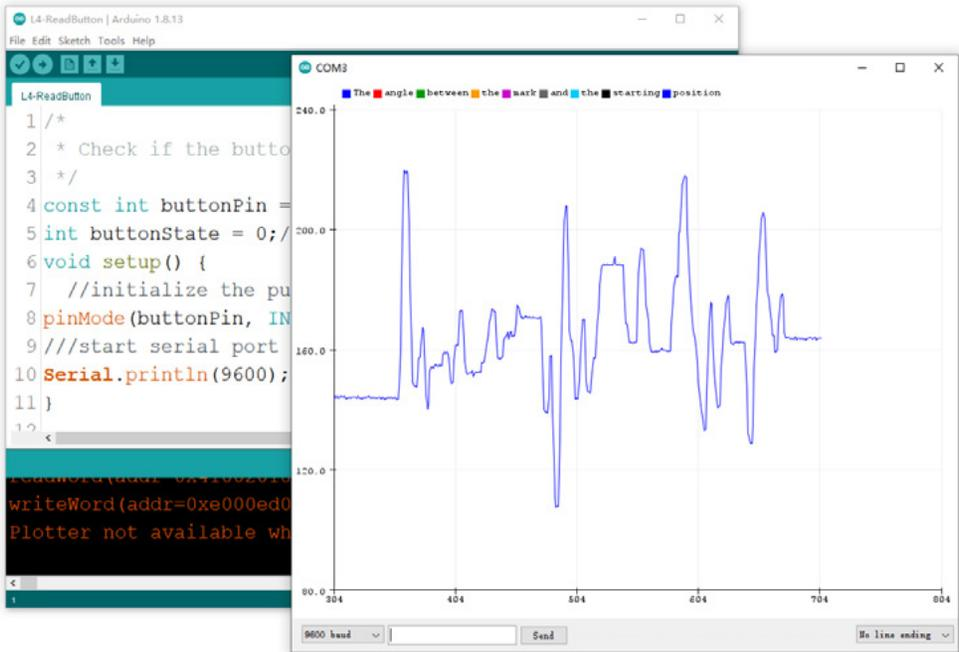
In the serial port plotter, the data acquired by the serial port will be plotted into an XY axis graph, where the X axis represents time, and the Y axis represents the data acquired by the serial port. Through the chart, we can see the change in the data more intuitively. Please try it.
