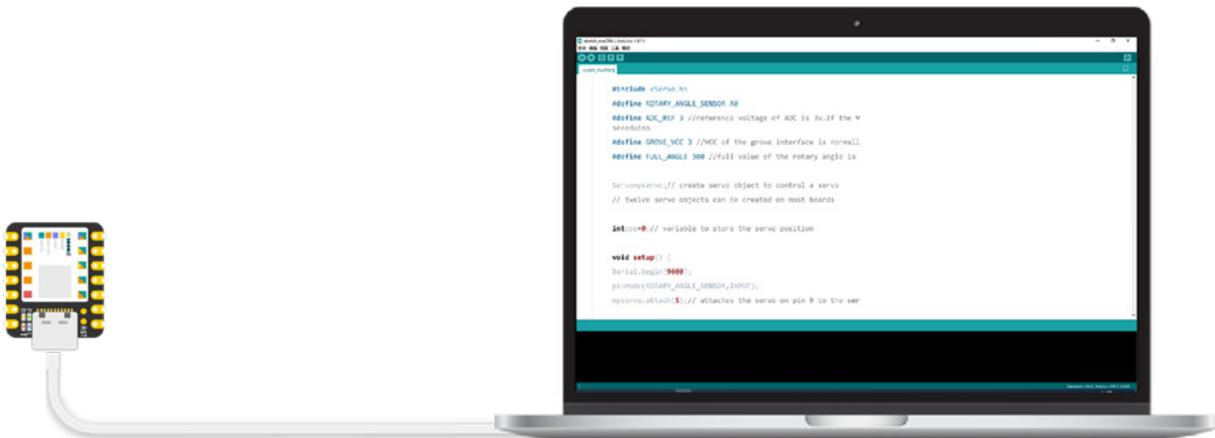
After installing the board, click **Tools** → **Board**, find “Seeeduino XIAO ” and select it. Now you have already set up the board of Seeeduino XIAO for Arduino IDE.
