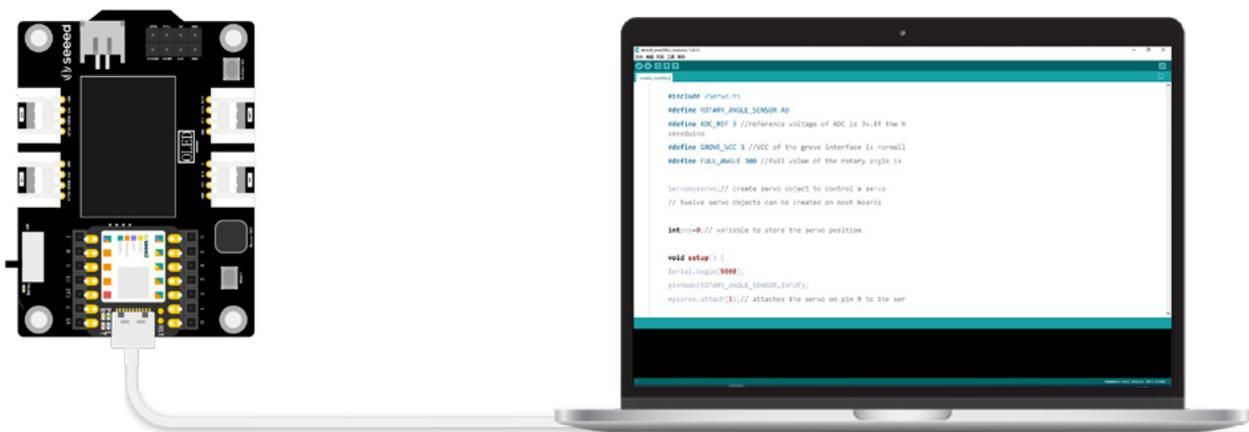
Next, click the “verification button” to verify the program.if the verification is correct, click the “Upload” button to upload the program to the hardware.When the debugging area shows “Upload Successful”,check whether there is a circular pattern on the OLED display.
