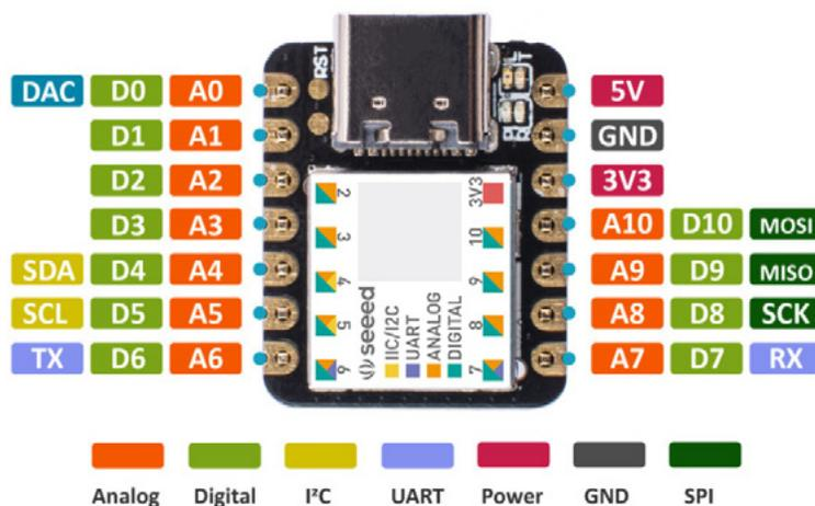
interfaces, 10 PWM interfaces (d1–d10), 1 DAC output pin D0, 1 SWD pad interface, 1 I2C interface, 1 SPI interface, 1 UART interface. We will introduce the functions of these pins one by one in the following study. Moreover, Seeeduino XIAO has a Type-C interface which can supply power and download code. There are two reset pads, you can short connect them to reset the board.
