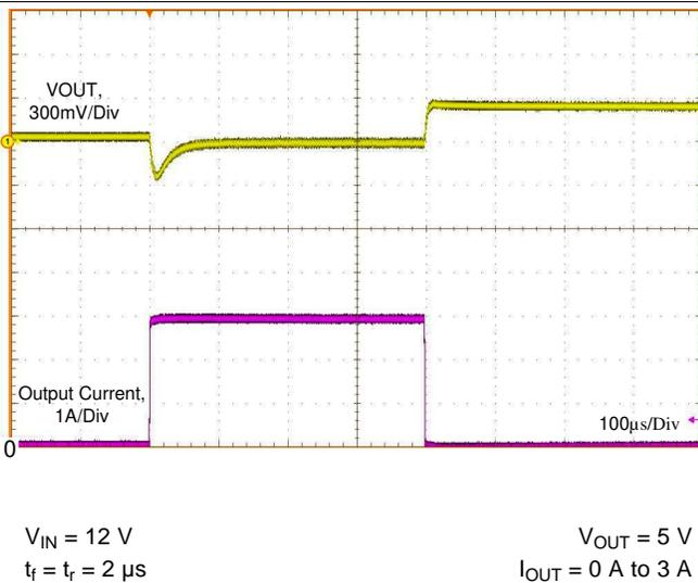
Figure 42. Load Transient
