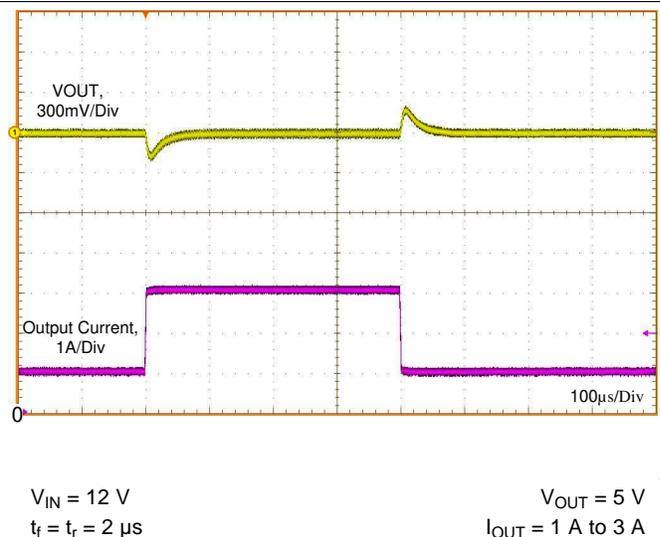
Figure 43. Load Transient
