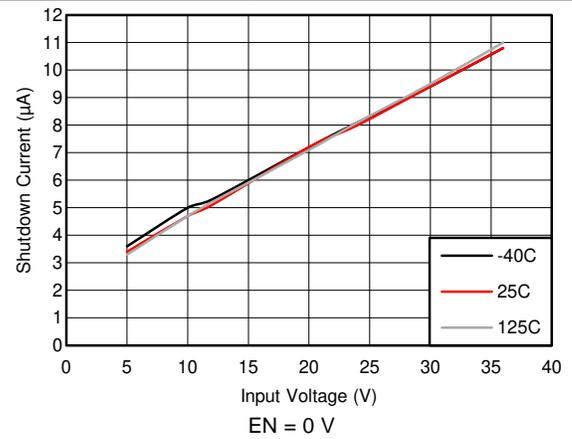
Figure 2. Shutdown Supply Current
