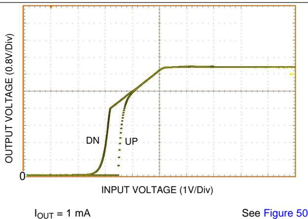
Figure 5. UVLO Thresholds
