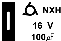
FRONT VIEW OF CAPACITOR
