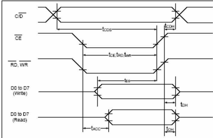
(  $V_{DD}=+5V\pm 5\%$ ,  $GND=0V$ ,  $T_a= -20$  to  $+70^{\circ}C$  )
