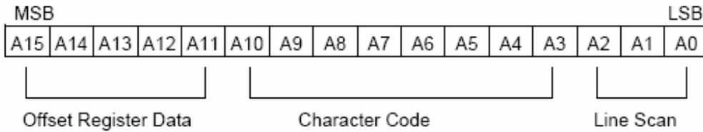
RA6963 assign External character generator, when character code set 80h to FFh in using Internal character generator. Character code 00h to 80h assign External character generator, when External generator mode
