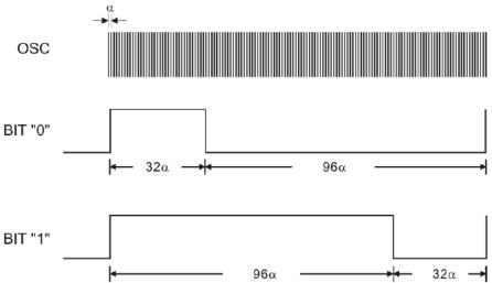
where the oscillating time period,  $\alpha = 1/f$  and (f is the oscillation frequency)
