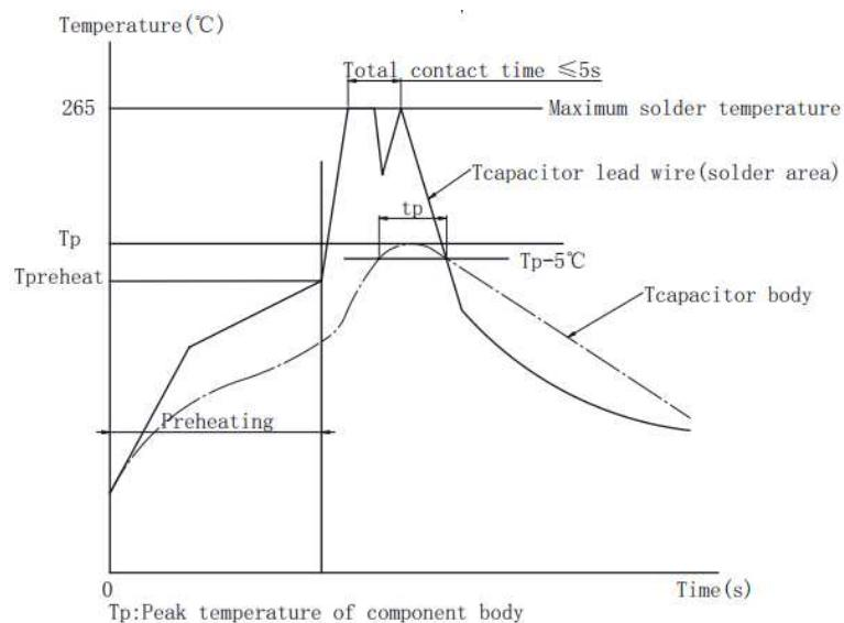
▲ Because overheating could damage the capacitor, we recommend paying attention to the maximum capacitor temperature and heating time, use temperature sensor to detect the maximum capacitor body temperature.
