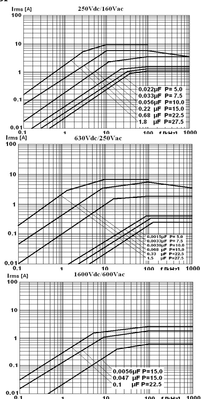
Note: sinusoidal wave-form, environment temperature  $\leq 85^{\circ}\text{C}$ , internal temperature rise  $\Delta T=10^{\circ}\text{C}$ , p (pitch) in mm.
