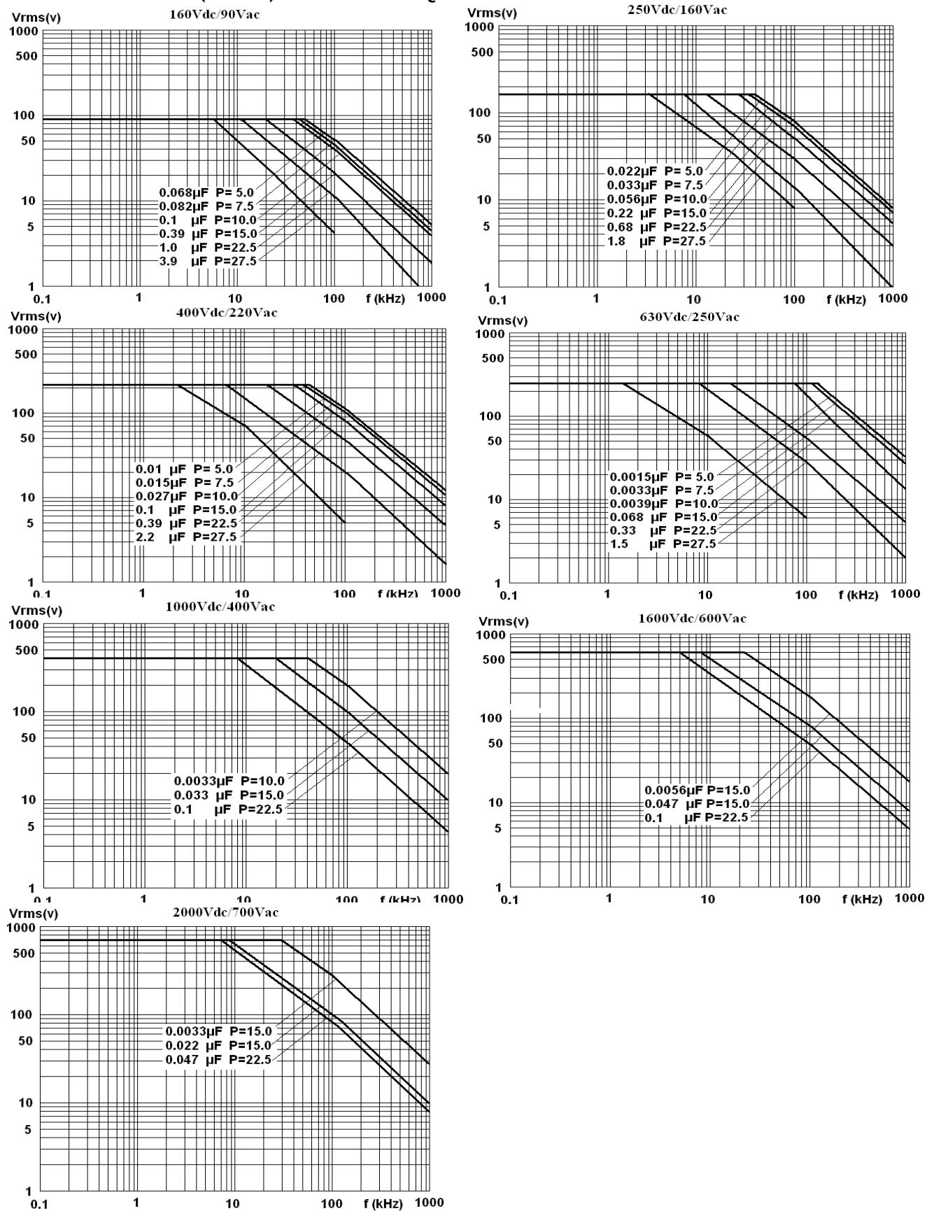
Note: sinusoidal wave-form, environment temperature  $\leqslant 85^\circ\text{C}$ , internal temperature rise  $\triangle T=10^\circ\text{C}$ , p (pitch) in mm..
