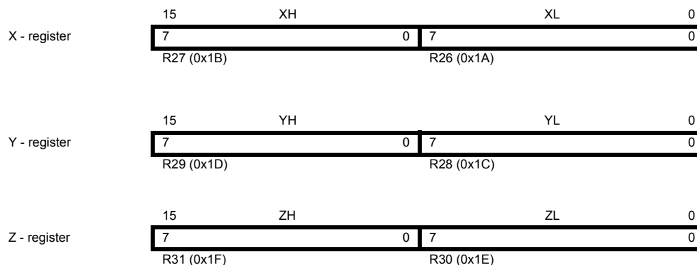
Figure 7-3. The X-, Y-, and Z-Registers
