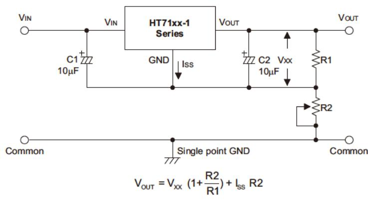
**Circuit for Increasing Output Voltage**
