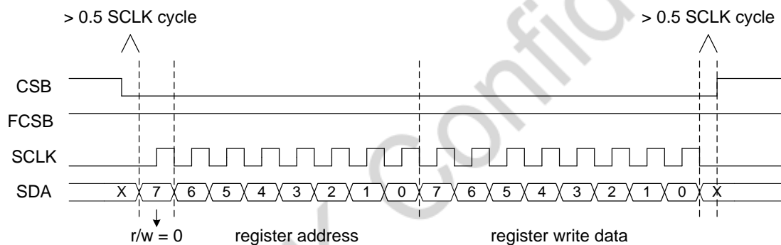
Figure 4-6. SPI write register timing
