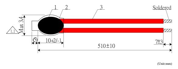
\*.THERMISTOR: T44S2101RP83003D COATING RESIN:BLACK EPOXY 2.LEAD WIRE:UL1332#30TS Red 3.TUBE:2.4mm KYNAR TUBE
