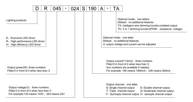
For example: DR045-024S190A-TA means: high performance LED driver; output power 45W; output voltage 24Vdc; output current 1900mA; single output; output voltage and current can be adjusted; with intelligent wire dimming function and isolated output.
