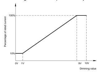
10V PWM signal for output current adjustment (Typical): Frequency range:100HZ ~ 3KHz
