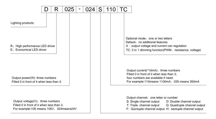
For example: DR025-024S110TC means it is a high performance LED driver, output power 25W, output voltage 24Vdc, output current 1100mA, single output, with intelligent wire dimming function and isolated output.
