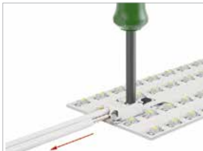
Inserting/removing fine-stranded conductors by lightly depressing the push-button (e.g., using the optional 206-861 Operating Tool).
