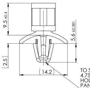
TO SNAP-LOCK IN A 4.75±0.08 DIA. HOLE, IN A 0.79-1.98 PANEL THICKNESS
